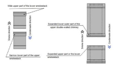
Fig.3. Assembling of the double-walled chimney
