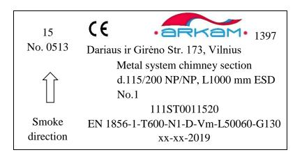
Fig.1.Example of identification of the elements of the double-walled chimney system
