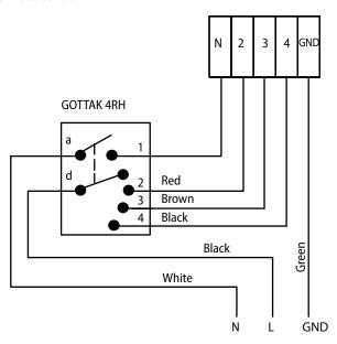
The circuit must include GCFI and overcurrent protection devices!
