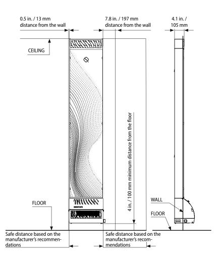
Figure 1B – Saunum AirSolo 70 / 80 model installation distances.
