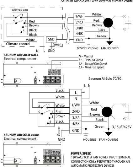
**Figure 6** – Wiring diagram: Air Solo, equipped with illumination and a switch.
