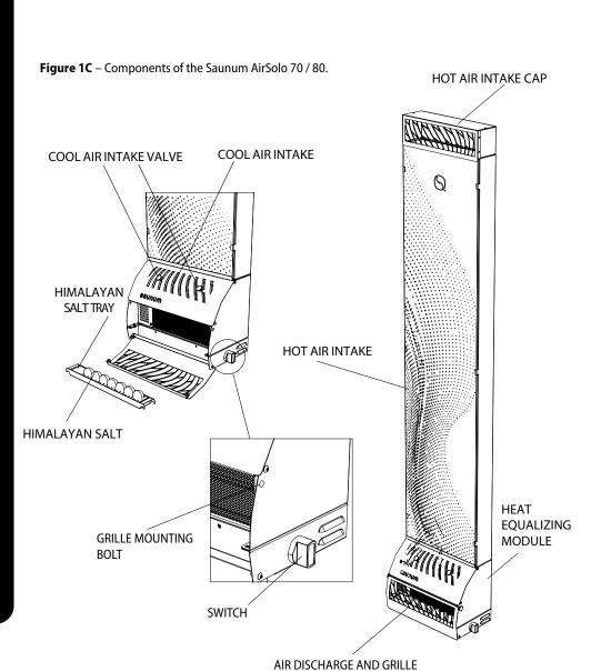
The Air Solo works most efficiently when the edge of the hot air intake opening is adjacent to the ceiling of the sauna room (model with a hot air intake cap). If the Air Solo is not equipped with a hot air intake cap, the Air Solo should be installed so that the upper edge remains 3–4 in. / 80–100 mm below the ceiling. The lower edge may not be closer than 4 in. / 100 mm. to the floor to prevent the water on the floor from coming into contact with the electrical wiring of the Air Solo.
