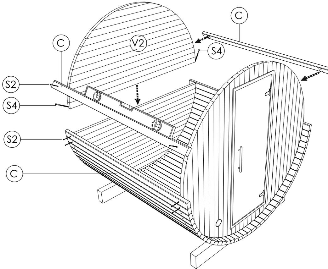
**STEP 8:** Continue placing body staves (C) tightly on both sides of the sauna using rubber mallet, and fixing body staves with screws 4.0x70(S2) . To finish the roof top joint, use roof finishing item (H). Different thickness filling peaces (H1)are provided to completely fill the gap.
