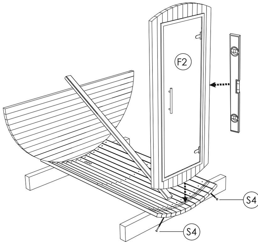
**STEP 6:** Attach side panel (F) using 4 5.0 x 120 (S4) screws. One person still holds door panel. Place body stave (C) on rear and front panel to connect both panels using 4.0 x 70 SS (S2) screws. Check panel level before fix them. These panels must be completely seated into the floor groove. Fix ventilation grill from inside on ventilation cuts.
