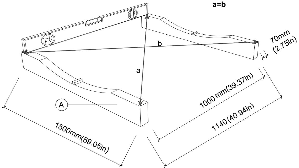
STEP 2: Place the support cradles (A) on level site. Carefully level for better stability. Place the center stave (B) on wooden dowels embedded in outer support cradles (A). Fix the center stave (B) with 5.0x100 SS(S1).
