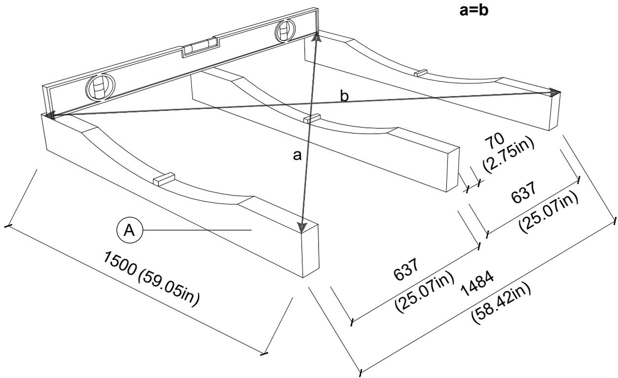
STEP 2: Place the support cradles (A) on level site. Carefully level for better stability. Place the center stave (B) on wooden dowels embedded in outer support cradles (A). Fix the center stave (B) with 5.0x100 SS(S1).
