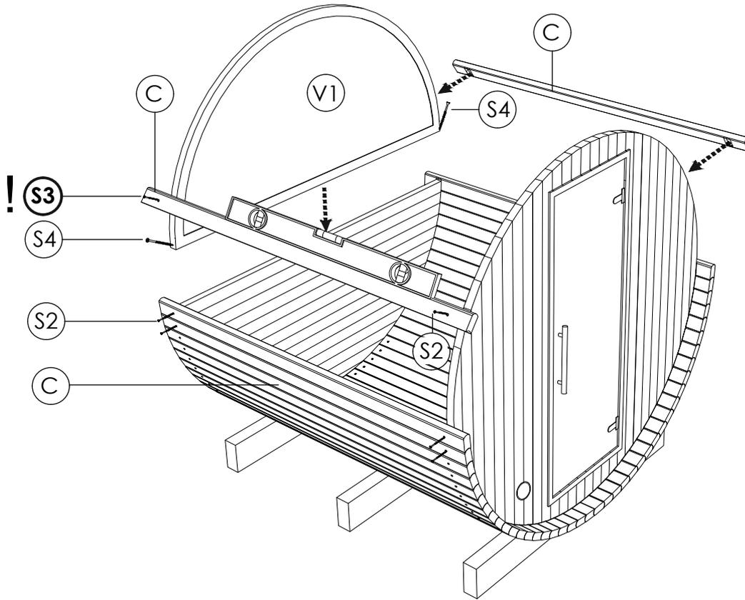
STEP 8: Continue placing body staves (C) tightly on both sides of the sauna using rubber mallet, while fixing body staves on the front panel with screws 4.20x70(S2) and rear window panel (V1) with fixing body staves on the front panel with screws 4.20x70(S2) and rear window panel (V1) with 4.0 x 50 screws (S3) to prevent glass breakage. To finish the roof top joint, use roof finishing item (H). Different thickness filling peaces (H1) are provided to completely fill the gap.
