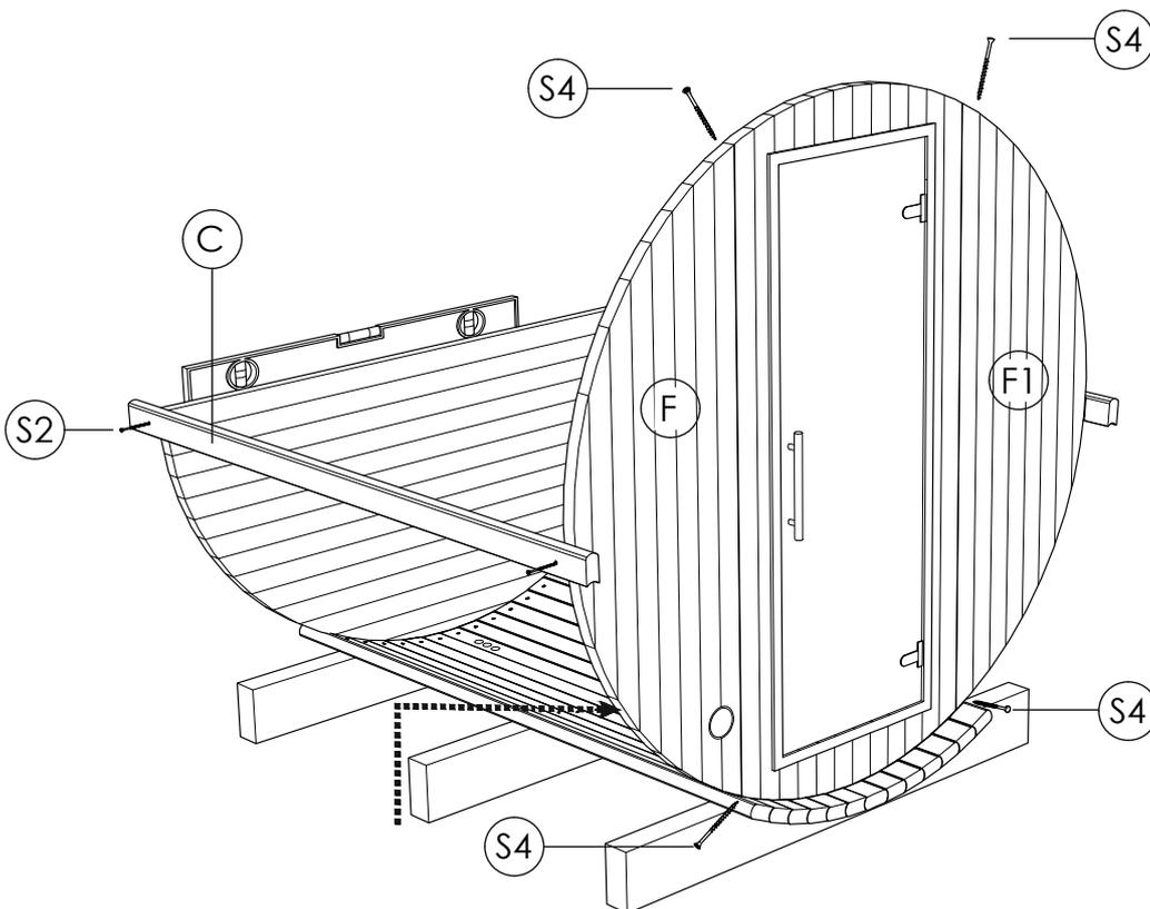
STEP 7: Place body staves (C) until the halfway point. Place rear panel with panoramic window (V1) on bottom rear panel (V), fix by 2 screws 5.0 x 120 (S4). Bind panels (F;F2; V1) together by temporarily placing two body staves (C) on each side.
