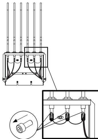
6. Undo the bolts holding the heating element module in place.
