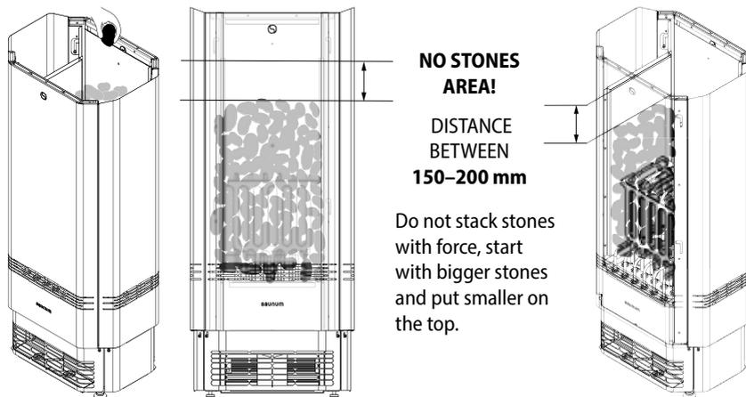
When you have filled the basket with stones like shown in graph, reposition the top grille and then add stones to it on and ensure that the air can move freely. Do not pile up and stack rocks on top of each other.
