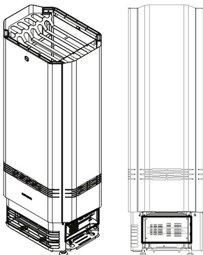
Do the electrical connections according to the schematic on page 30. Feed the cable through the openings in bottom of the heater near the cable terminals.
