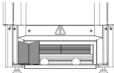
After moving the air deflector to the desired position, add 2 Himalayan saltball and reposition the bottom front panel.
