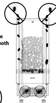
**NOTE! Do not drop any stone inside of the both side flue!!!**
