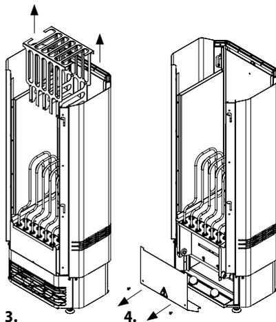
4. Remove the panel covering access to the heating elements. Undo the two bolts holding it in place
