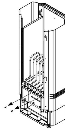
**NB! Each heating element is fixed with special gaskets, star-washers and nuts.**
