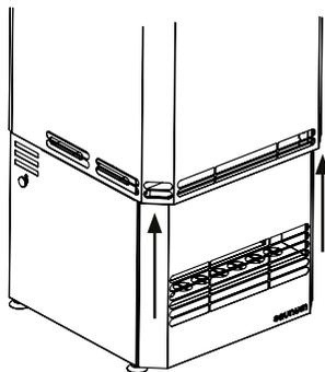
Pull from under the output grille edge outwards.
