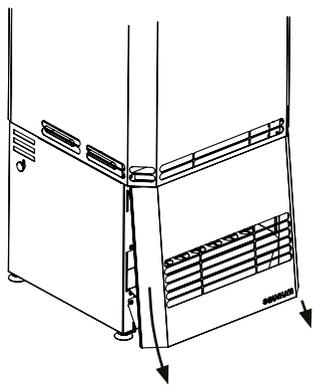
Remove the output grille by holding it slightly tilted and pulling it downwards.
