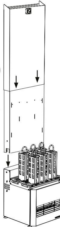
2. Place the parts of the hot air intake inside each other. Next, place the lower part of the intake at the end of the heater's intake socket and adjust the feet of the heater; check the intake and the housing to make sure the device is level. Adjust the heater housing as needed.
