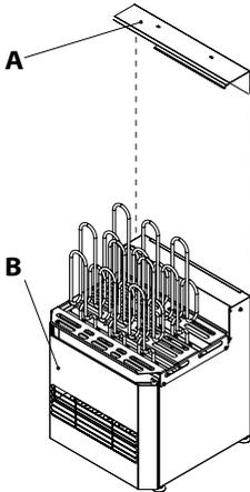
Place the cap at the connection point between the wall and the ceiling (corner) and fasten with a mounting suitable for the base material. It can be attached to the wall and/or the ceiling. Center the heater under the cap and adjust the feet so that the device is level.
