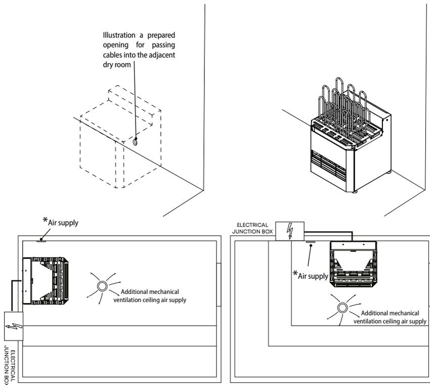
\* Recommended location of the air supply hole. Exact location may change according to the size and shape of the room.
