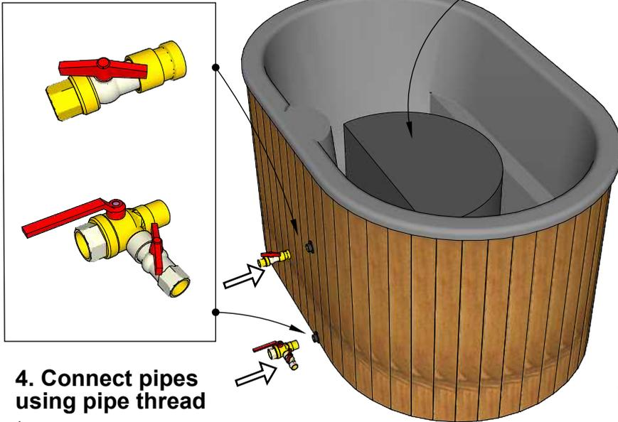
4. Connect pipes using pipe thread tape.
