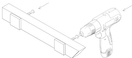
The raised parts on the outer edges of the supports enable ventilation between the wall and the sauna bench module.
