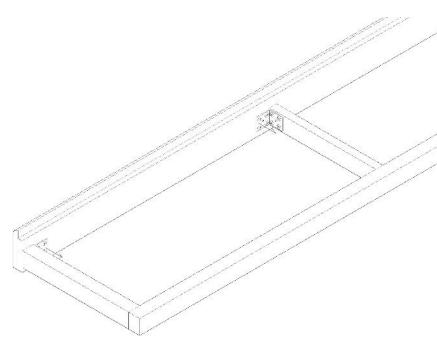
On modules 90 and 108, the frontboard is screwed directly onto the frame
