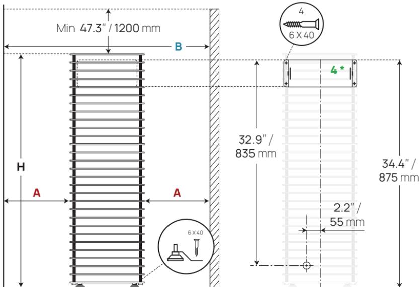
\* CLIFF Mini 4 is attached to the wall with a special bracket
