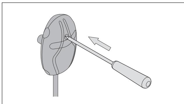
**Figure 10.** Reset button of the overheat protector
