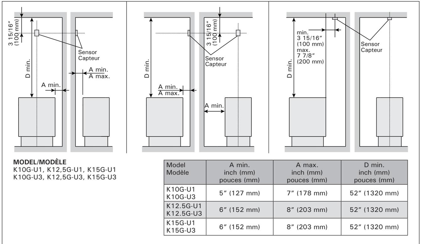
**Figure 7. The place of the temperature sensor of the control unit in connection with floor-mounted heaters**
