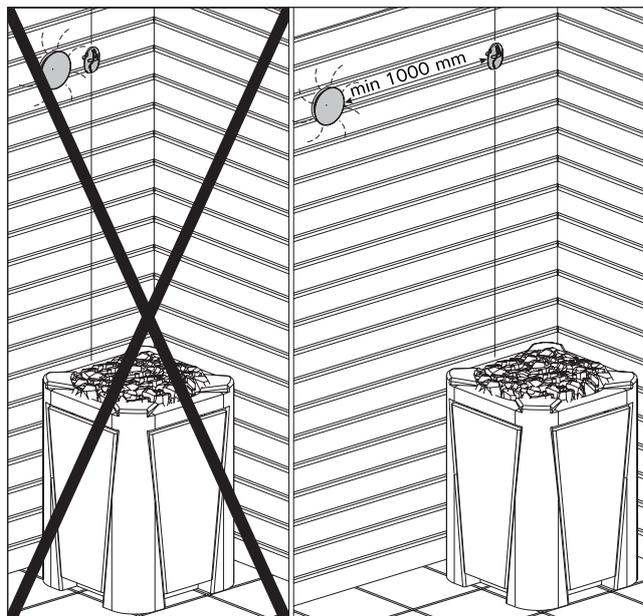
**Figure 9.** Sensor's minimum distance from an air vent
