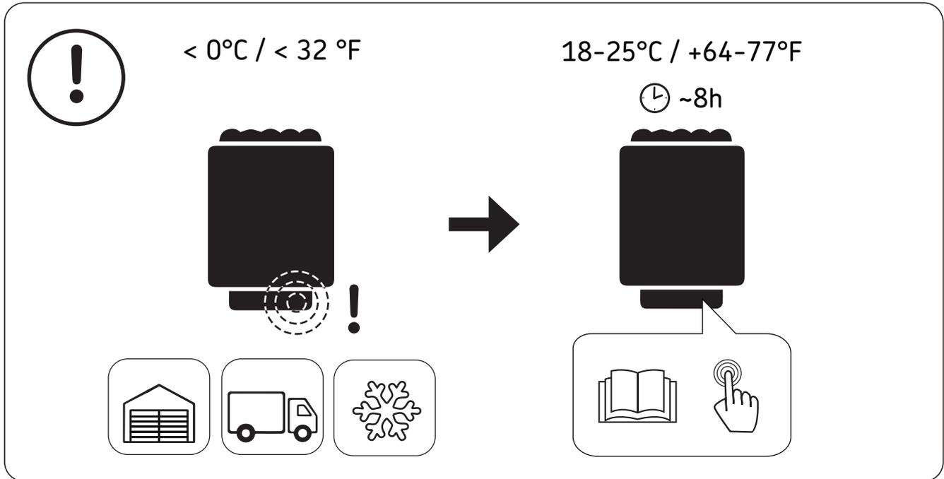
**!** Overheat protector of the device can go off also at temperatures below -5°C / 23°F (storage, transport, environment). Before installation take the device to the warm environment. The overheat protector can be reset when the temperature of the device is approx 18°C / 64°F. The overheat protector must be reset before using the device. See the user manual > Resetting the Overheat Protector.
