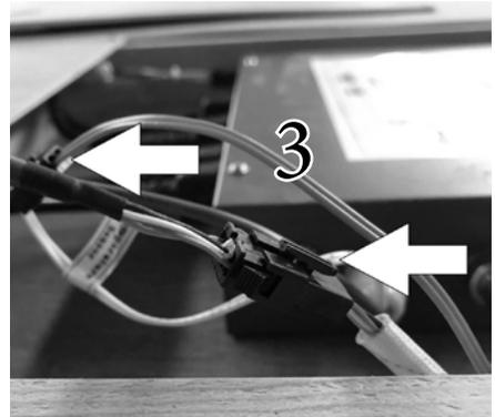
4. Plug the power cable into the power supply.
